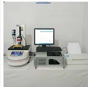
3. Load Curve Meter
