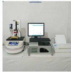
3. Load Curve Meter
