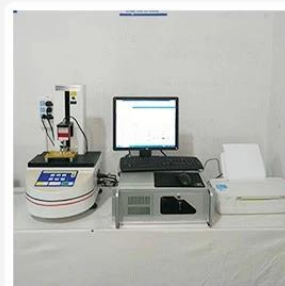
3. Load Curve Meter
