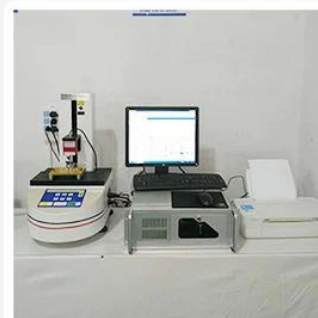
3. Load Curve Meter
