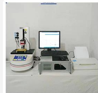
3. Load Curve Meter
