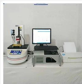
3. Load Curve Meter
