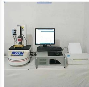
3. Load Curve Meter
