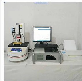
3. Load Curve Meter
