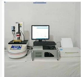
3. Load Curve Meter
