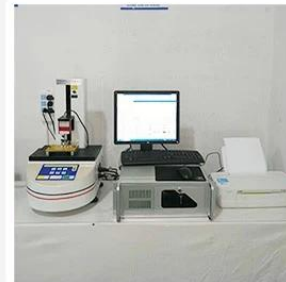
3. Load Curve Meter
