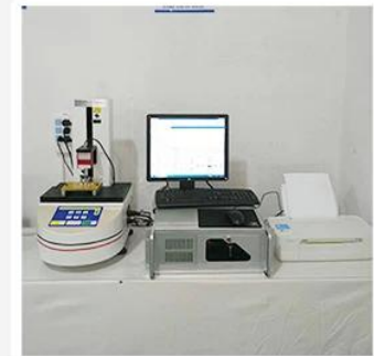
3.Load Curve Meter
