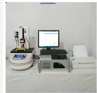
3. Load Curve Meter
