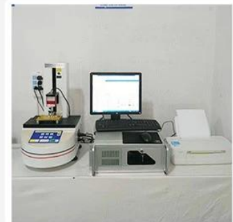
3. Load Curve Meter
