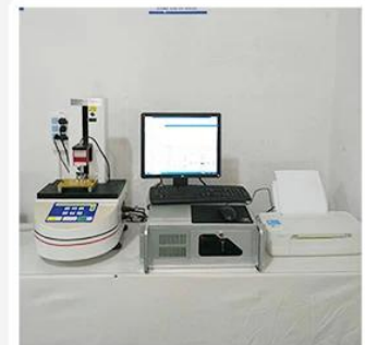
3. Load Curve Meter
