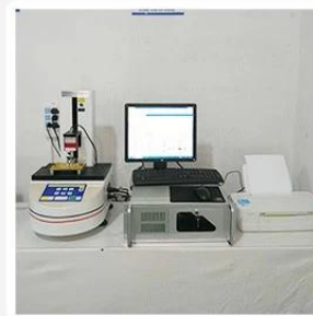
3. Load Curve Meter
