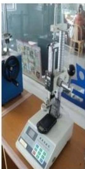
A white spring tester with a digital display and a control panel, used for testing springs.                  |
