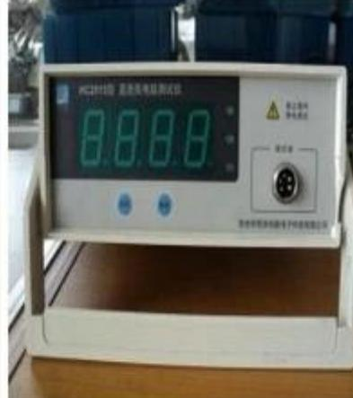
A white digital current resistance tester with a large green LED display showing '8888' and a warning symbol. |
