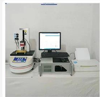
3. Load Curve Meter
