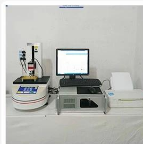
3. Load Curve Meter
