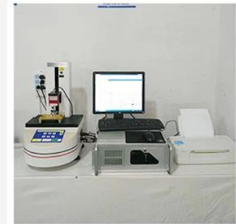
3. Load Curve Meter
