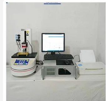
3. Load Curve Meter
