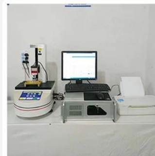
3. Load Curve Meter
