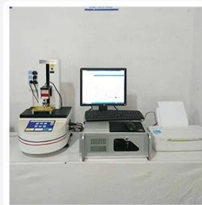
3. Load Curve Meter
