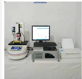
3. Load Curve Meter
