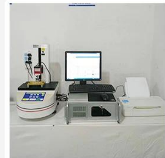
3. Load Curve Meter
