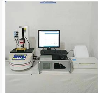
3. Load Curve Meter
