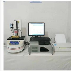
3. Load Curve Meter
