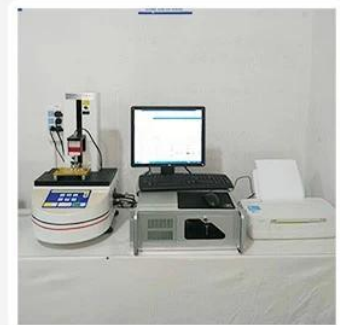
3. Load Curve Meter
