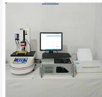
3. Load Curve Meter
