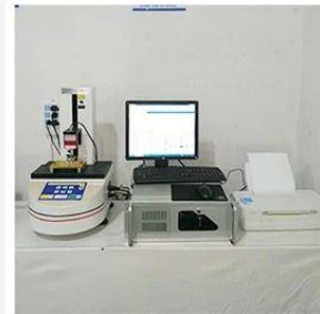
3. Load Curve Meter
