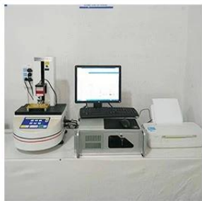
3. Load Curve Meter
