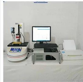
3. Load Curve Meter
