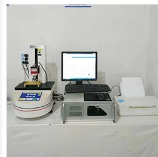
3. Load Curve Meter
