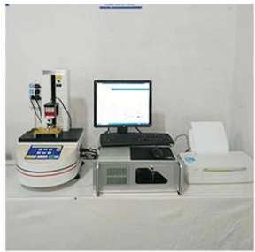
3. Load Curve Meter
