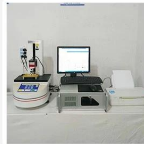
3. Load Curve Meter
