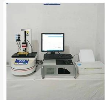
3. Load Curve Meter
