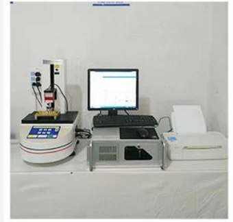
3. Load Curve Meter
