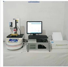
3. Load Curve Meter
