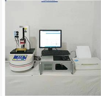
3. Load Curve Meter
