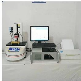
3. Load Curve Meter
