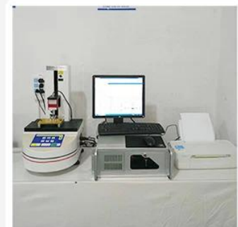
3. Load Curve Meter
