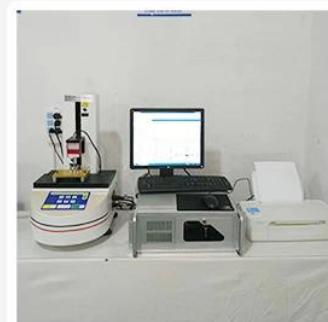
3. Load Curve Meter
