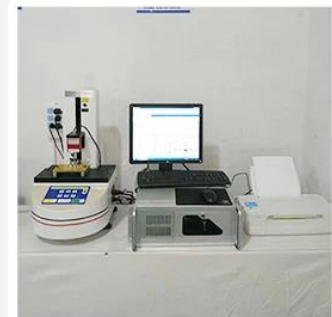
3. Load Curve Meter
