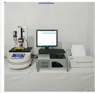
3. Load Curve Meter
