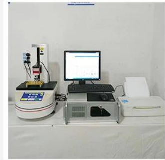
3. Load Curve Meter
