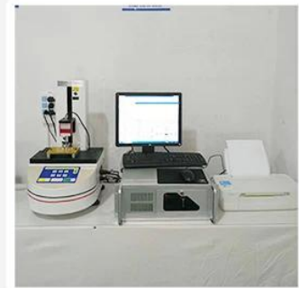
3. Load Curve Meter
