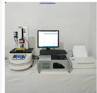
3. Load Curve Meter
