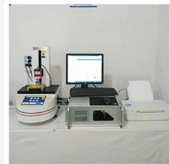
3. Load Curve Meter
