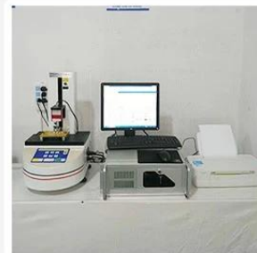
3. Load Curve Meter
