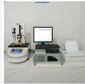
3. Load Curve Meter
