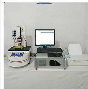
3. Load Curve Meter
